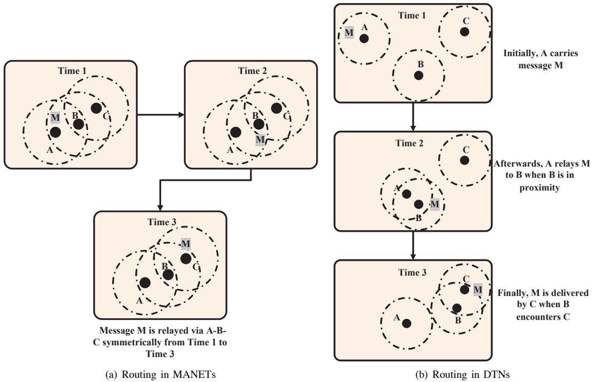
Fig. 2. Illustration of Routing in MANETs and DTNs
