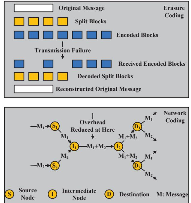
Fig. 8. Difference Between Erasure Coding and Network Coding
