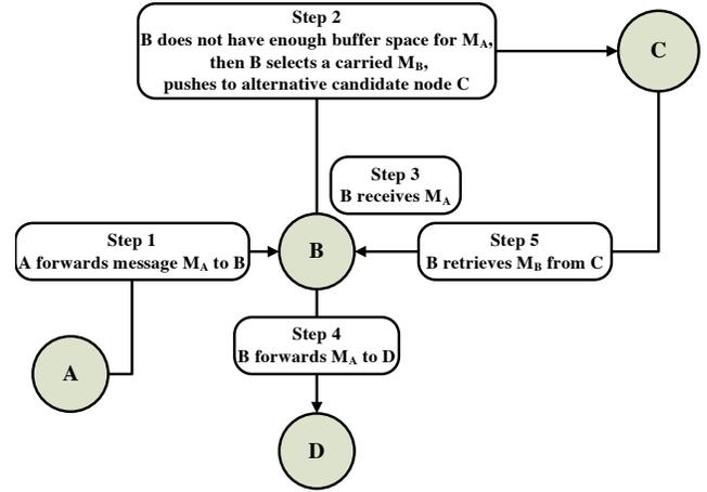
Fig. 10. Congestion Control Process of the Works in [43][44]
