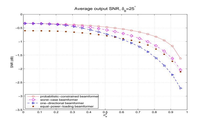
Average SNR vs. error variance  $\sigma_e^2$ . Correlated fading with angular spread  $\delta_{\theta} = 25^{\circ}$ .
