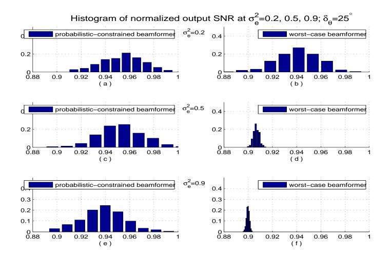
Histogram of normalized SNR for  $\sigma_e^2 = 0.2, 0.5, 0.9$ . Correlated fading with angular spread  $\delta_{\theta} = 25^{\circ}$ .
