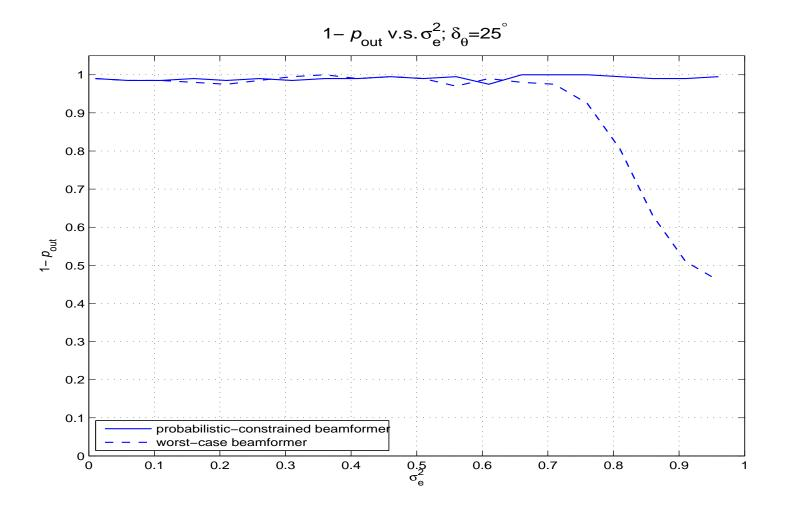
$(1 - p_{out})$  vs error variance  $\sigma_e^2$ . Correlated fading with angular spread  $\delta_{\theta} = 25^{\circ}$ .
