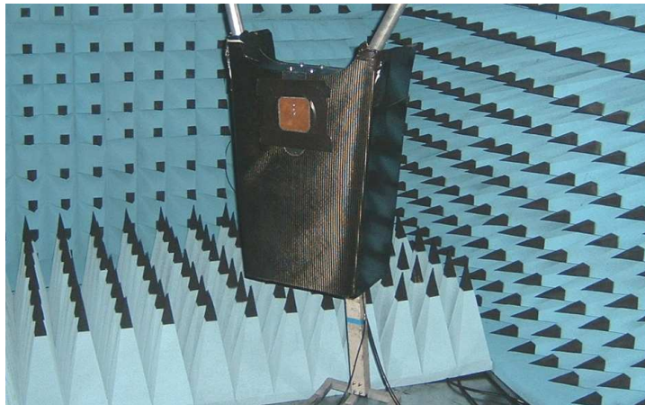
Conformal vehicle-mounted antenna under testing
